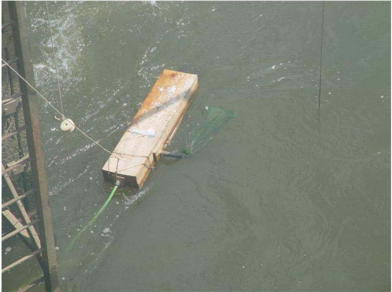
Figure 2. Photo of an Irish Elver Ramp used to sample elvers (young American eels) at the base of Conowingo Dam during 2005.
