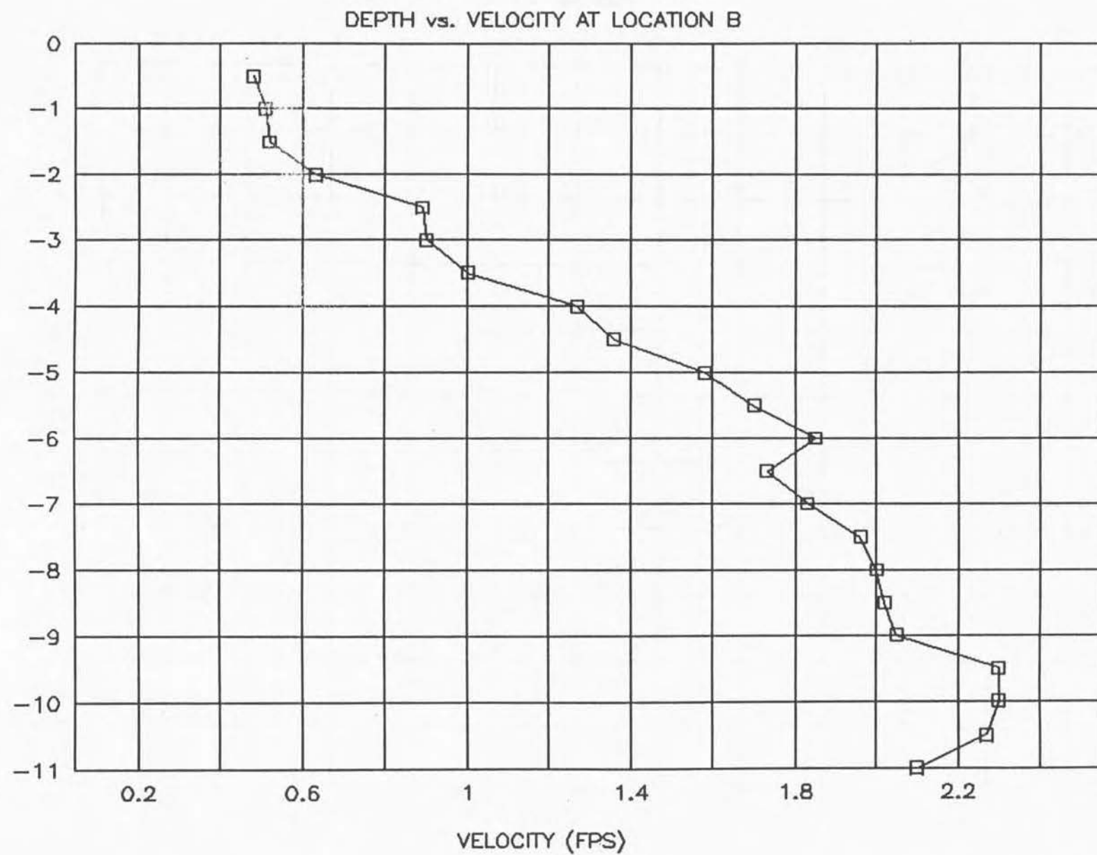
FIGURE 8 SKIMMER WALL VELOCITY MEASUREMENTS HOLTWOOD HYDROELECTRIC PROJECT
