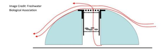
Silo Design: A concrete dome forms the outer structure, providing protection and stability. A PVC chamber is placed inside the dome, creating a smaller, controlled environment for the mussels. The PVC chamber is often covered with a mesh screen to allow water flow and prevent mussels from escaping.
