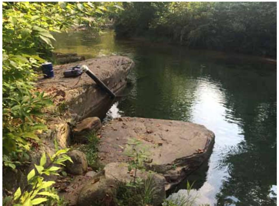
*Data sonde at Pleasant Creek, Lycoming County, Pa. The data sonde is a multi-parameter water quality sonde with optical dissolved oxygen and turbidity probes, a pH probe, and a conductance and temperature probe. The data sonde also includes a non-vented relative depth sensor. The entire unit is placed in protective housing and secured in free-flowing water at each site.*
