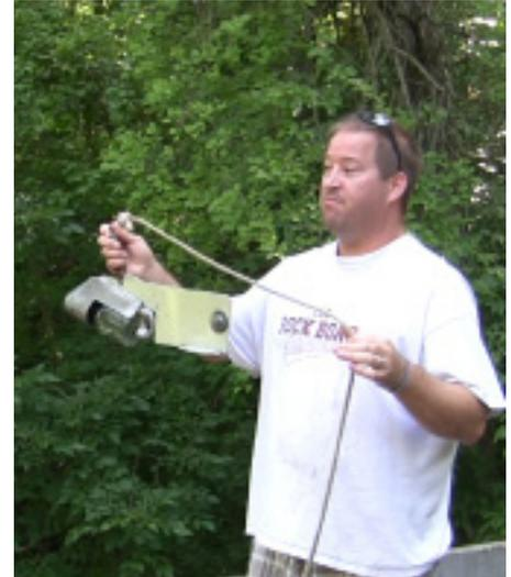
SRBC Environmental Scientist Kevin McGonigal displays USGS depth integrated sampler used to collect water that is analyzed for Total Nitrogen, Total Phosphorus, Total Organic Carbon, and Suspended Sediment.
