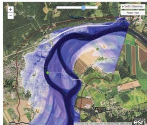
*Inundation map for Jersey Shore, PA. Light blue areas indicate possible water levels at flood stage.*
