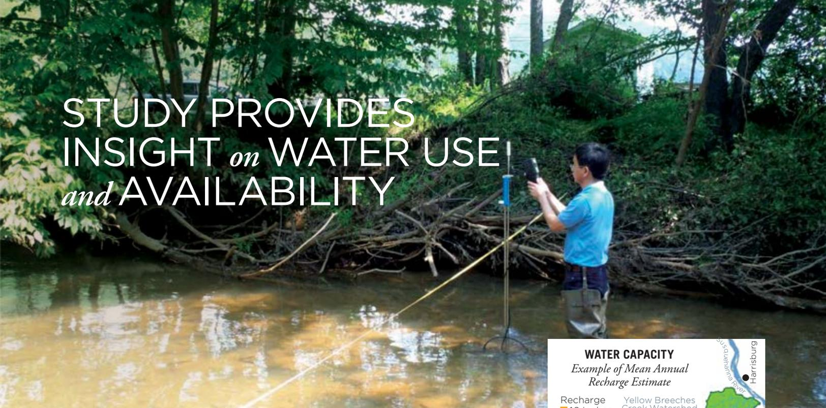
Staff measuring streamflow during stable conditions.
