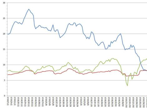
Figure 2. Continuous monitoring results of temperature (blue line), pH (red line), and dissolved oxygen (green line) from July – Oct 2013 on the Susquehanna River at Kirkwood, NY.
