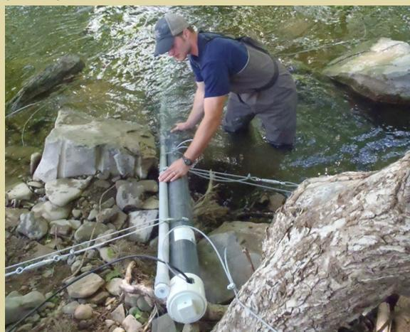
*Monitoring instruments must stay submerged even during low flow conditions and be placed deep enough to stay below the ice during winter. There should be enough flow to prevent leaves and sediment from building up around the sonde.*
