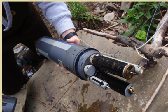
*At each station, a water quality sonde (above) is secured either to the stream bottom or contained within a PVC casing secured to the streambank (below).*
