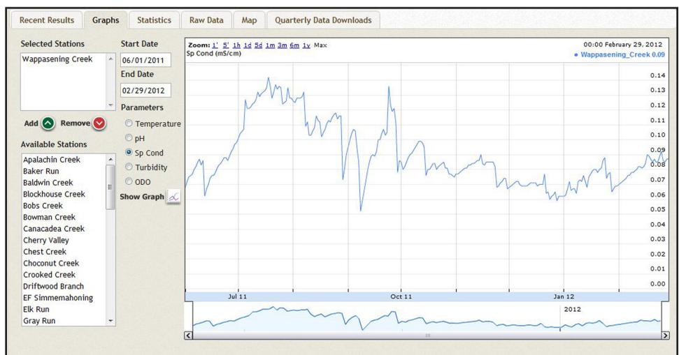
Graph showing Specific Conductivity at the Wappasening Creek station from June 2011 through February 2012. Elevated levels of conductance in water can be a leading indicator of impacts from natural gas activities.
