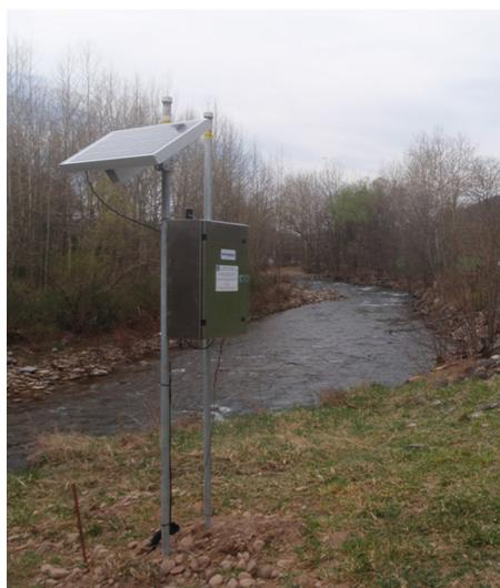
*The data platform is powered by a rechargeable 12V battery connected to a solar panel.*
